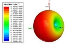
Fig. 5: Simulated 3D model of total gain in (dB) of the proposed antenna printed on RF4 Antenna
