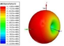
Fig. 7: Simulated 3D model of total gain in (dB) of the proposed antenna printed on PET film Antenna
