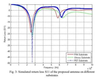
Moreover, annealing and multilayer printing technique causes a wideband antenna, as shown in Fig. 3. Such flexible multilayer wideband antenna is suitable to operate at several bands of different wireless communication systems.
