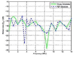
Fig. 4: Measured return loss S11 of the proposed wideband antenna on different substrates
