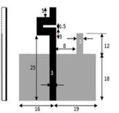
Fig. 1: Geometry of antenna front and back side
