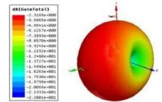
Fig. 6: Simulated 3D model of total gain in (dB) of the proposed antenna printed on Glossy Antenna
